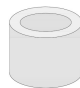
Image 20– Example of metal bushing that should be used to make the fixed points when the holes on the panels are all made with the same diameter as for the sliding points.
