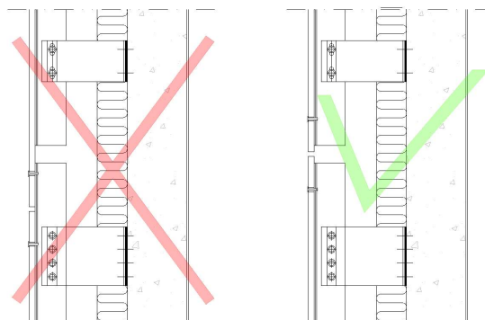
Image 8– Vertical sections – Examples of incorrect and correct arrangement of cladding panels along an expansion joint between one subframe vertical profile and the next
