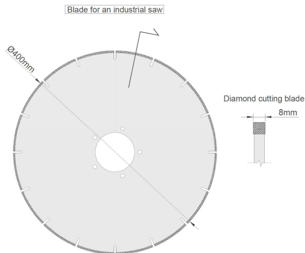
Image 46 – Example of a blade used to cut the panels at the Società Italiana Lastre Srl plant
